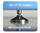
optical surfaces and automatically compensates to provide a correct measurement in real time. Conversely, the NanoDrop™ One stretches the sample column to 1.0 mm and only alerts the user to a sample column anomaly and does not report a measurement result.
